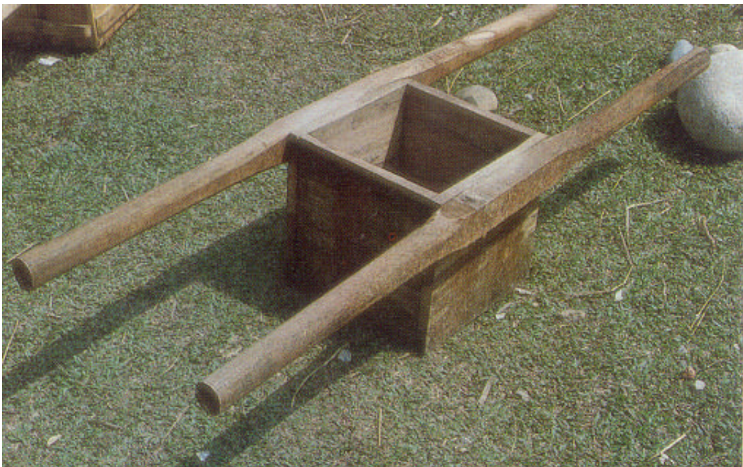
Photo 8. Gauging Box to ensure delivery of correct volume of Aggregate for each batch.
